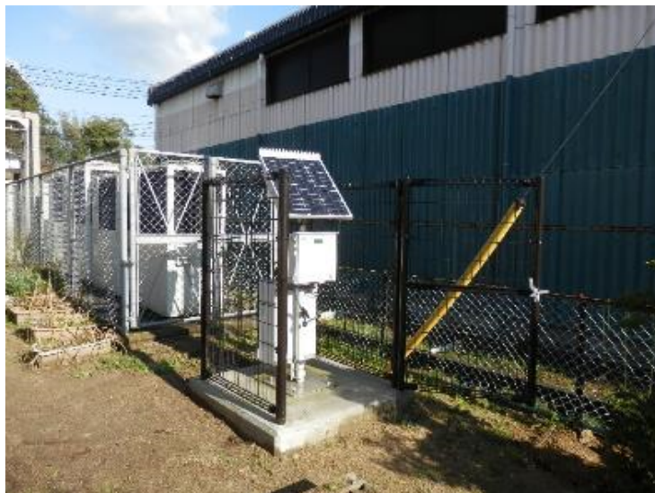
Figure 5.5 Example of the installation status of a simplified electronic dosimeter (Shimane Prefecture)
