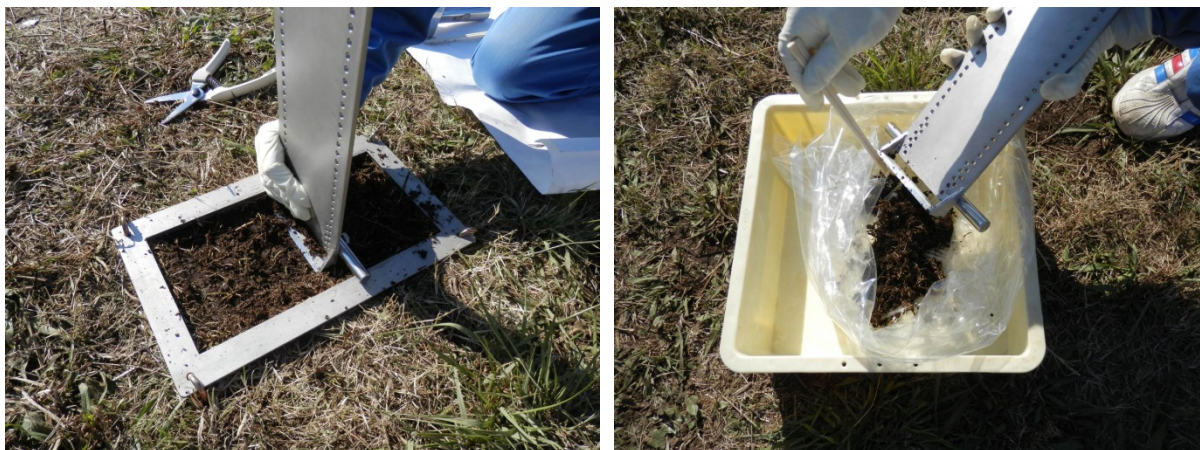
Figure E.7 Soil sampling using a scraper plate
