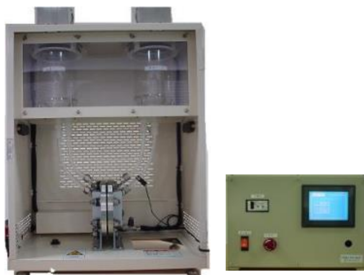
Figure 2.8 Schematic of the solid polymer electrolytic enrichment device
