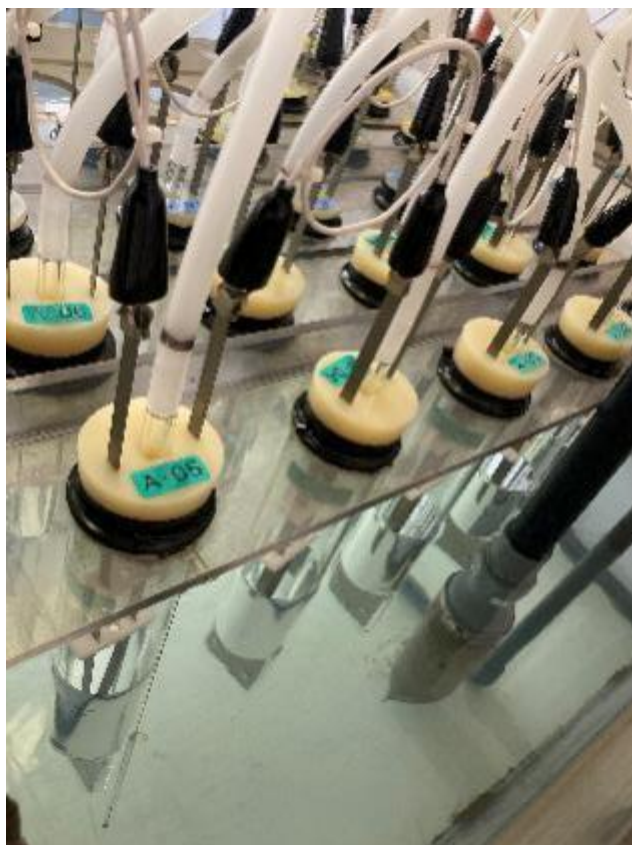
Figure 2.6 Electrolytic enrichment with metal electrodes
