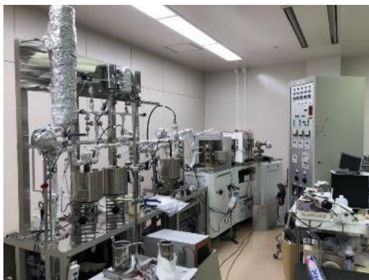
Figure D.3 Noble-gas mass spectrometer (Gas purification line in the front and mass spectrometer in the back)
