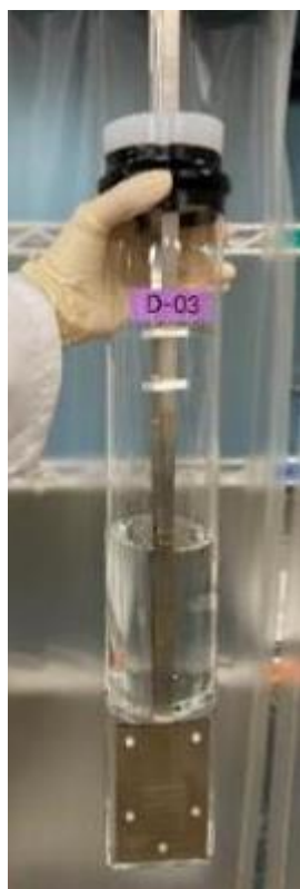
Figure 2.5 Electrolysis cell for electrolytic enrichment with metal electrodes (before electrolysis)
