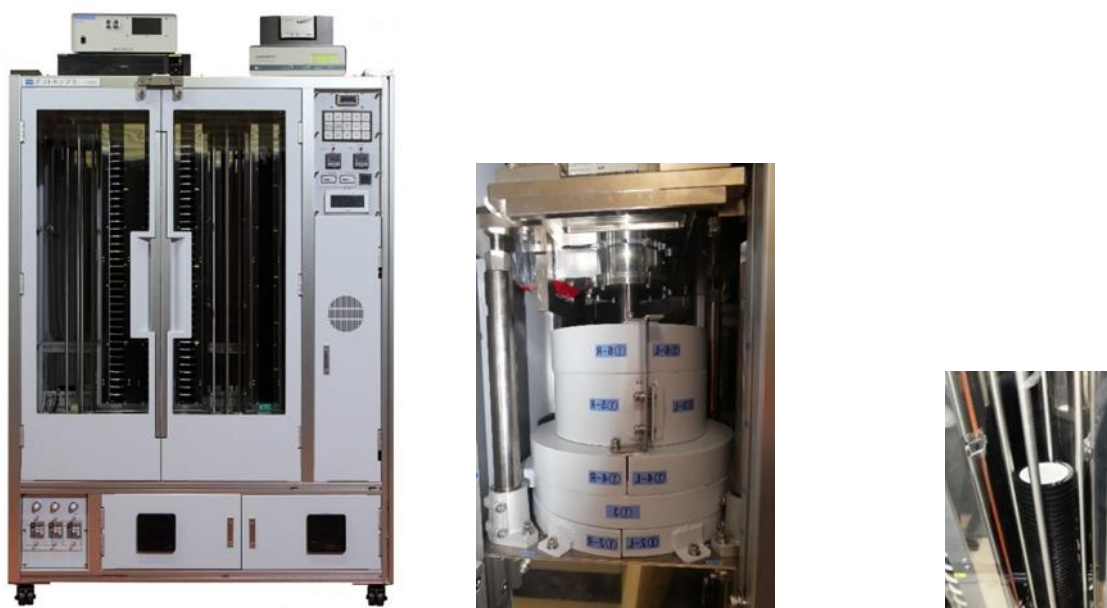
Figure Information C-6. Example of dust monitor using a germanium semiconductor detector
