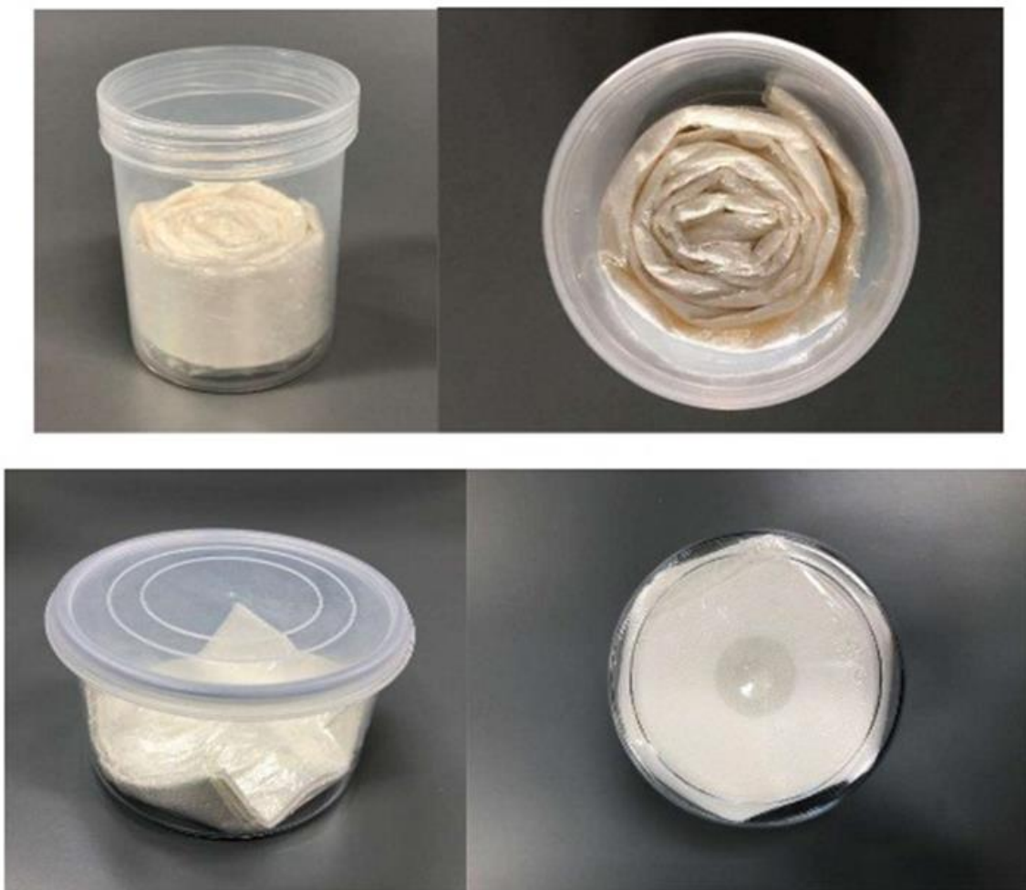
Figure 4-4. Example of filling long filter paper (78 mm x 700 mm) used for 6 hours (Top: An example of filling a U-8 container with filter paper folded long and narrow so that the air sampling surface is close to the bottom. Bottom: Example of filling a V-9 container by overlapping and folding it for each hour so that the air sampling surface is centered)
