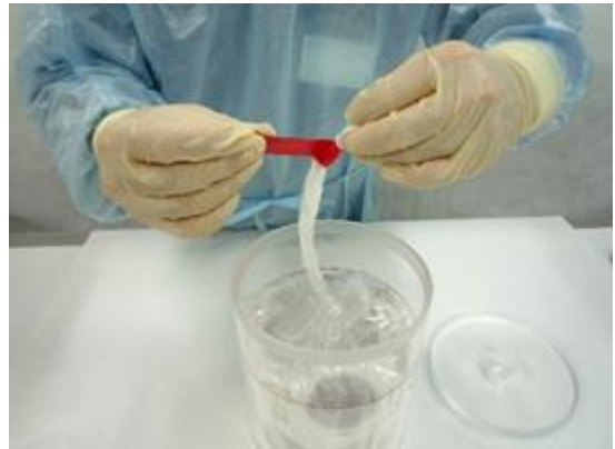
Photo 6.5. Closing the inner bag with plastic tape (long filter paper)
