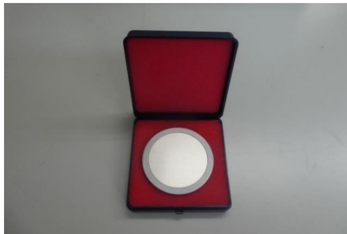
Figure 3-2. Example of standard source (Cl-36, 2-inch \phi )
