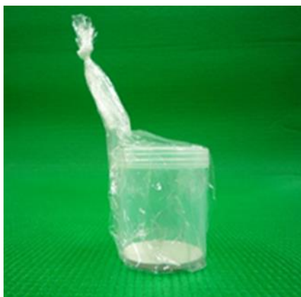
Photo 6.3. Example of a small container (glass fiber filter paper) covered with a polyethylene bag
