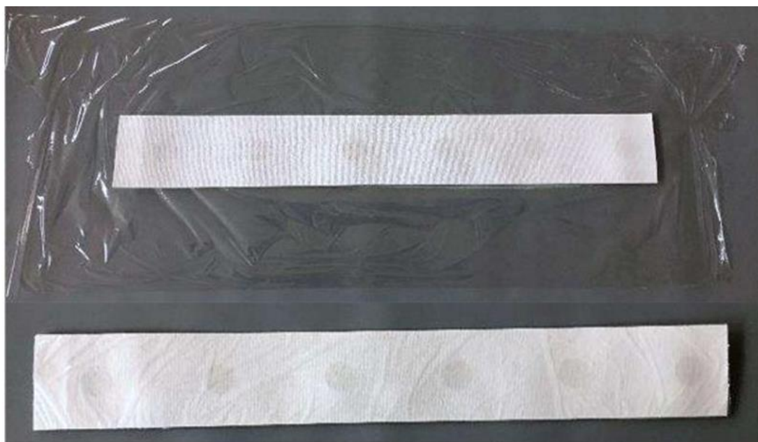
Figure 4-3. Example of long filter paper wrapped with polyethylene film, etc. (Top - before wrapping, bottom - after wrapping)
