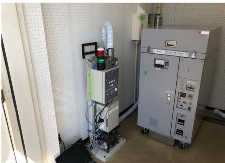
Figure Information B-1. Dust monitor used for comparative measurement
