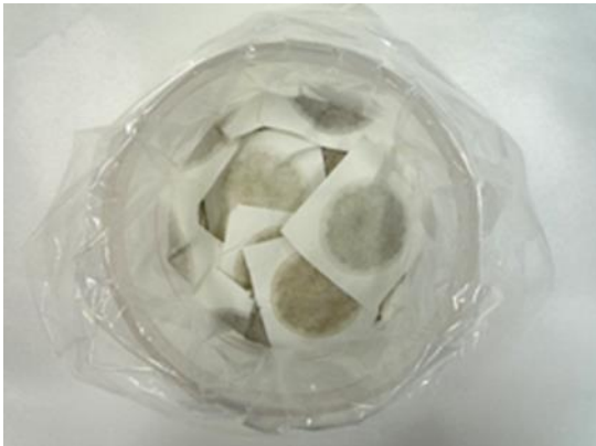
Photo 6.4. Filling a sample into a Marinelli container (long filter paper)
