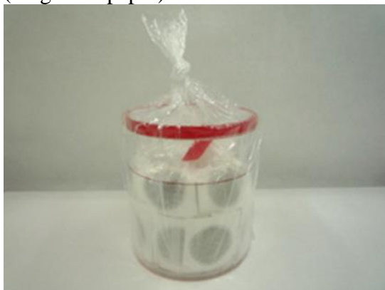
Photo 6.8. Marinelli container (long filter paper) covered with a polyethylene bag
