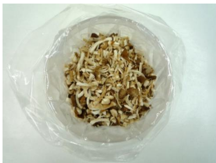
Photo 2-21 Sample packed inside the Marinelli beaker (Shiitake mushrooms)
