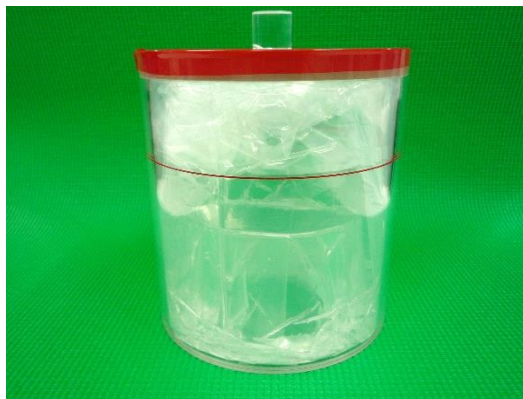
Photo 2-11 Fixing the lid with a plastic tape
