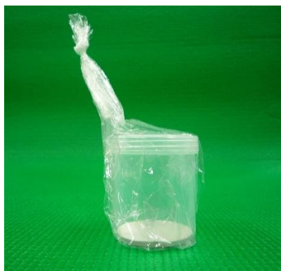
Photo 2-6 Small containers covered with a polyethylene bag
