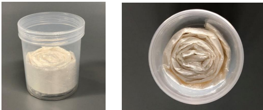
Photo 2-7 Example of placing a long roll paper cut into six-hour portions (Example of a roll packed into a small container and folded to make a long strip so that the dust collecting surface is close to the bottom)
