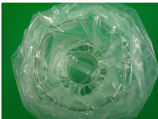
Photo 2-8 Filling a sample into the Marinelli beaker
