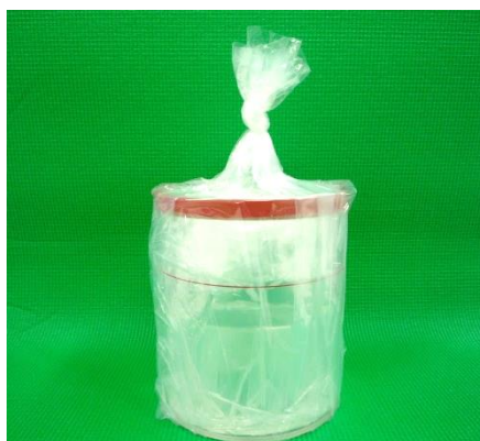
Photo 2-12 Marinelli beaker covered with a polyethylene bag
