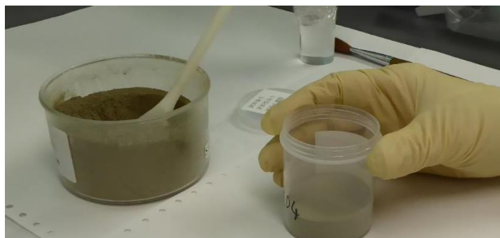
(e) Put the sample in the measuring vessel by dividing into several batches.
