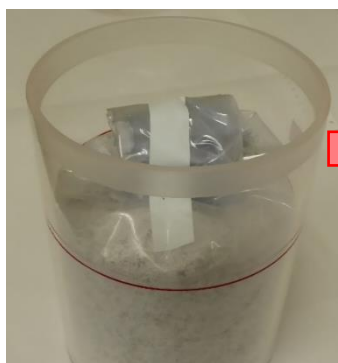
(f) Close the inlet of the inner bag and cover it with the lid.
