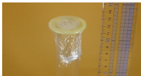
(c) Cover the pressing surface of the sample filling tool with a polyethylene sheet
